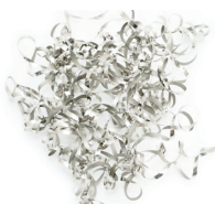
Chips generated by conventional cutting
