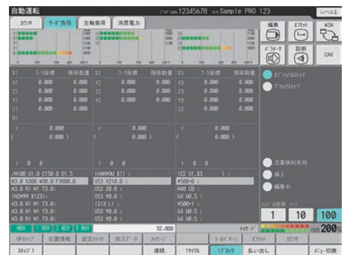
Automatic operation screen Motor load information is displayed graphically, allowing intuitive status checks.
