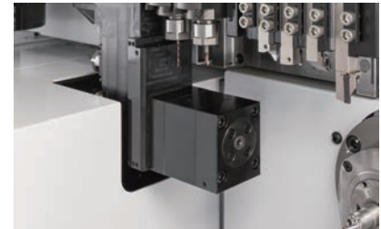
During B-axis tool change
