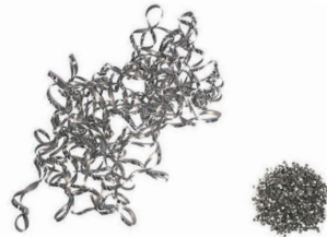
Chips generated by conventional cutting Chips with LFV
